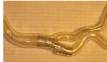
Figure 2: silicon mock carotid artery with the implantation of a stent
